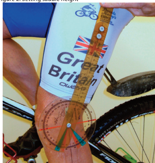
Figure 2: Setting saddle height
